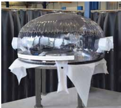
Fig 8. Medium size standard enclosure showing large entry zip, two sets of glove ports and a posting port.
