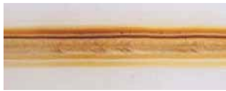
Weld made with 70 ppm oxygen in purge gas
