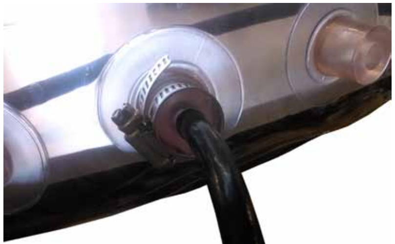
Fig 7. Glands for electrical, weld torch and water feed through.
