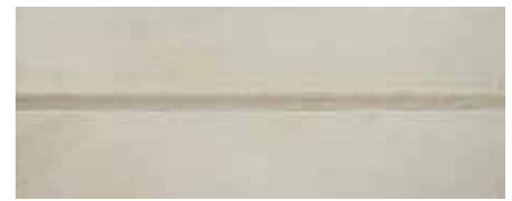
Weld made with 12 ppm oxygen in purge gas
