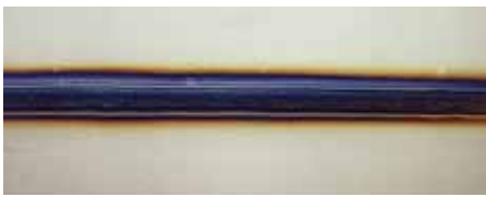
Weld made with 500 ppm oxygen in purge gas
