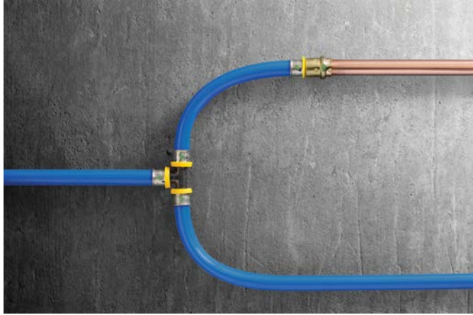
Photo 2-3: Viega copper to PEX transition fittings enable running large mains in copper and transitioning to PEX tubing up to 2" diameter for branch runs.
