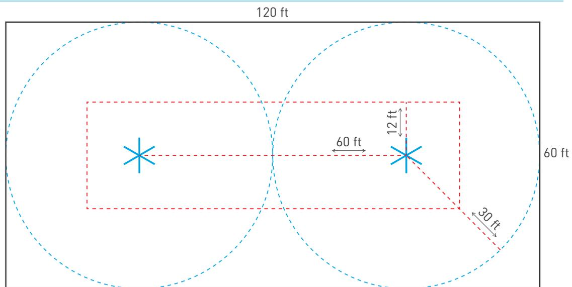
This diagram shows the proper spacing for two 8-foot HVLS fans. The fans are 60 feet apart. The smaller rectangle shows the minimum space required for an 8-foot HVLS fan (12 feet from the wall) and the large rectangle shows the maximum coverage radius.
