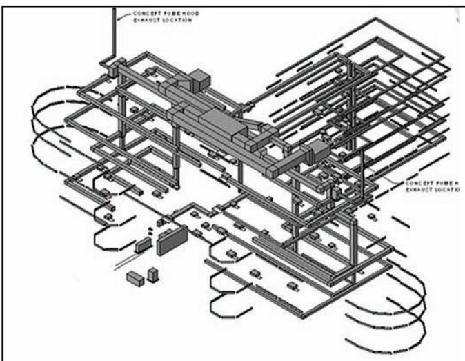
On the 1100 Broadway project, the Glumac team used their BIM-based design model to quickly perform “what-if” analyses for an under floor air system versus a traditional overhead system—quantifying for both the architect and the building owner the energy and cost savings.
