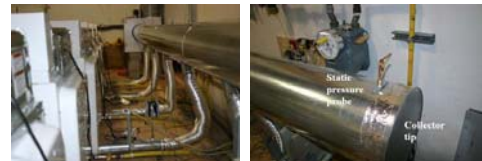
Fig . 7: Test system setup
